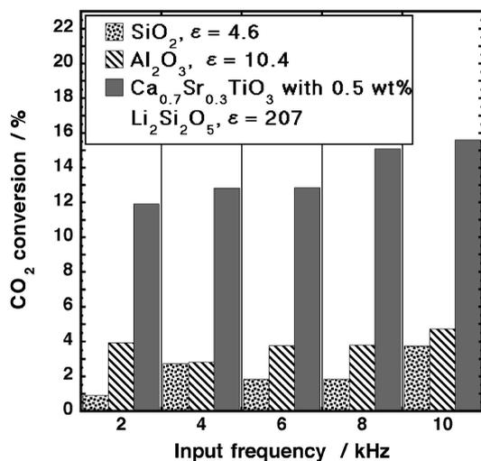
**Figure 2.** Input frequency dependence of  $\text{CO}_2$  conversion using different dielectric barriers (their permittivities are shown in the legend).
